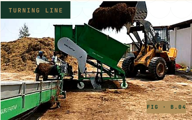
Loader-fed turner — 54-tonne cycle per shift.
